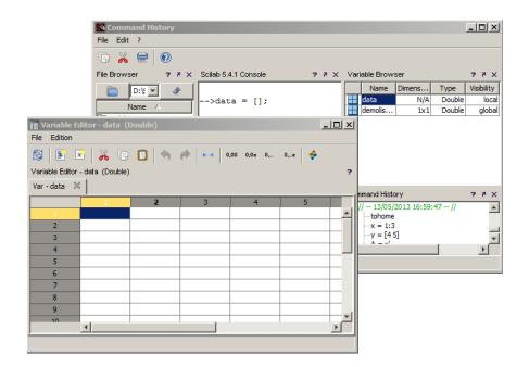
We now paste in the table given by the Variable Editor the data copied from Excel (figure on the right), making the variable "data" available in Scilab for data processing. We can paste the data from the clipboard.
