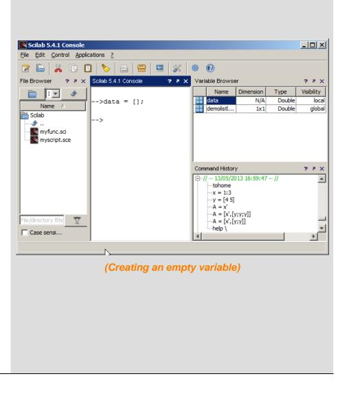
Once our variable has been created, it is possible to select in the Variable Browser the cell "data" with a double click, which will open the **Variable Editor**, as shown in the figure below.
